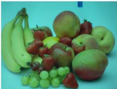
LCD technology demonstrating colour decay after 3,470 hours of operation
