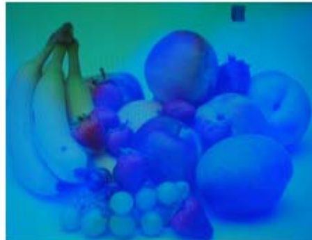
LCD technology demonstrating colour decay after 3,470 hours of operation
